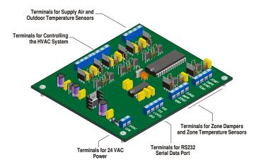
The residential Zone Control Module is similar to the commercial except it does not have the all the features. This module can control two zone dampers and a single or two-stage HVAC system. The control provides the same energy savings as the commercial version.
