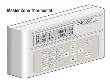
The Master Zone Thermostat provides a means of programming the Zone Control Module and displaying data from the module. The Master Zone Thermostat (MZT) has a 2 line by 16 character LCD display, a keyboard for entering, displaying and retrieving data and an RS232 communications interface for communicating with the Zone Control Module.
